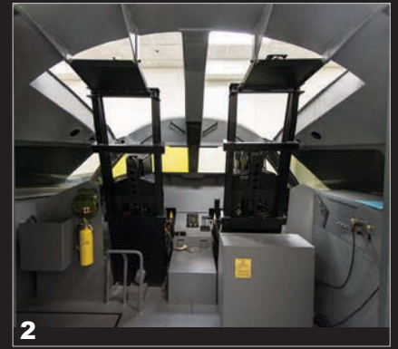
/1/ The Air Force named most B-2s after states, along the lines of the old Navy battleships. Here, AV-16, Spirit of Hawaii, is illuminated by ceiling lights in its custom hangar (both front and back doors are open for engine runs). /2/ The B-2 egress trainer gives pilots periodic refreshers in how to exit the airplane in an emergency. It can be filled with smoke and has all the lights and caution signals of a real cockpit. That training was used only once, in 2008, when the B-2 Spirit of Kansas crashed in Guam. The pilots survived a low-altitude ejection without major injury. /3/ Air traffic control apprentice A1C Chanel Johnson checks the runway from Whiteman's tower. /4/ Call sign Dexter, the supervisor of flying, acts as the operations group commander's eyes and ears in the tower, monitoring weather and area flight ops. /5/ Spirit of Hawaii looms in its hangar. /6/ During an annual inspection, Spirit of Alaska has its stealth materials scrutinized by techs from the 509th Maintenance Squadron and the 131st Maintenance Squadron, an Air National Guard unit. On the fuselage are SSGt. Joshua Fleshman (left) and A1C Steven Sahn.
