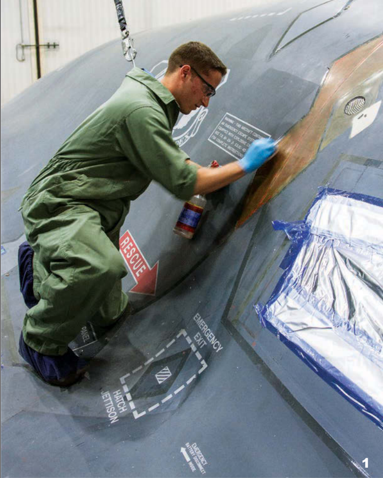
/1/ Sahd, a low observables tech with the 131st, applies stealth coatings. Note his boot covers, protecting the B-2's stealth finish. For large applications and repair, Whiteman has a specialized stealth coatings facility. /2/ The B-2s share Whiteman with A-10s of the 442nd Fighter Wing, an Air Force Reserve unit. /3/ The 394th's T-38s are serviced under sun shades on the tarmac. /4/ Spirit of Indiana and a T-38 chaser make a low sunset pass over Whiteman.
