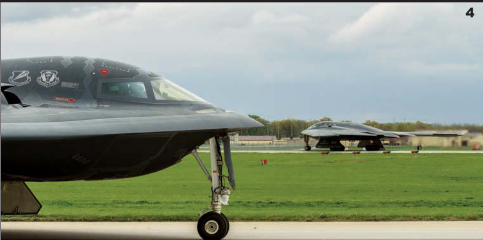
/1/ Spirit of Indiana lowers its landing gear. Having no vertical control surfaces, the B-2 relies on deflecting its tail/wing flaperons for yaw control. Seen deflected at the aircraft's rear, they can also function like a speed brake. Computers make the split-second calculations needed to keep the B-2 stable in flight. /2/ SrA. Steven Lee of the 309th Operations Support Squadron adjusts an oxygen mask for a waiting pilot. /3/ A1C Jared Schanen of the 509th OSS performs maintenance on a parachute to be carried in a T-38 ejection seat. /4/ Spirit of Indiana taxis as Spirit of Missouri, in background, starts down Runway One at Whiteman. /5/ Above the Truman Military Operating Area, a pair of 394th T-38s fly in formation.
